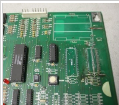
This MPU sustained alkaline damage. Sockets for the 68B09E processor and the 6264 RAM have been removed.
