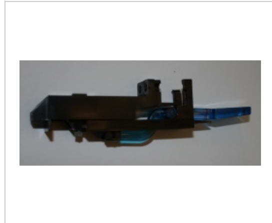
The first step to disassemble a target. Slide the rear face of the target assembly up.
