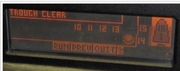
A Stern Monopoly in "Clear Ball Trough" Mode Identifying One Ball in the Trough
