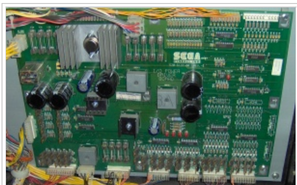
Stern White Star I/O Power Driver Board
