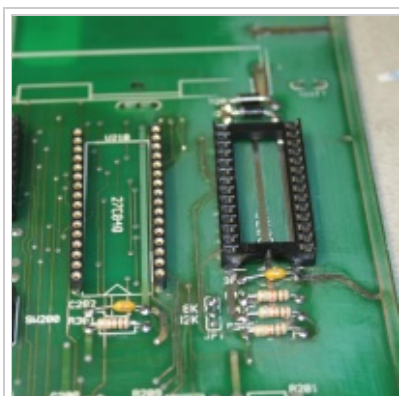
Bare copper traces tinned.
