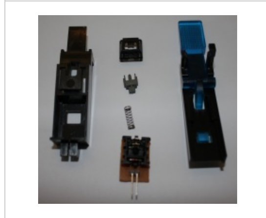
"Exploded" target parts. The gray switch part must be oriented correctly. Note the integrated diode just under the micro-switch, center/bottom.
