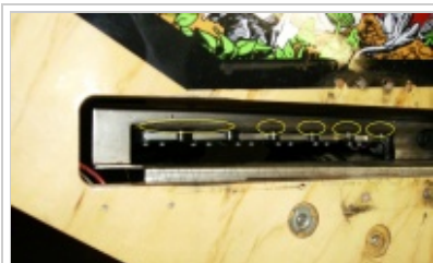
Ball trough assembly with divots. Although it's not a White Star game, Jurassic Park is used for this example.
