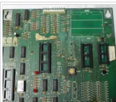
The aftermath of batteries which leaked. This board is beyond repair, and good only for salvage parts.
