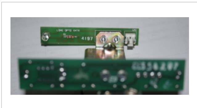
The opto transmitter side.
