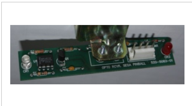
The opto receiver side, with accompanying electronics. The red colored LED is a diagnostic aid to indicate a detected switch closure.
