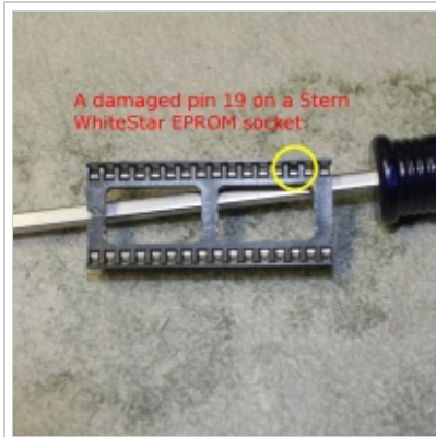
A damaged EPROM socket from a Sega/Stern White Star MPU
