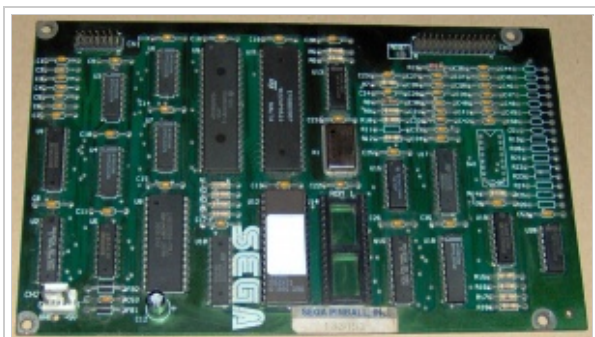
Sega White Star Display Controller Board
